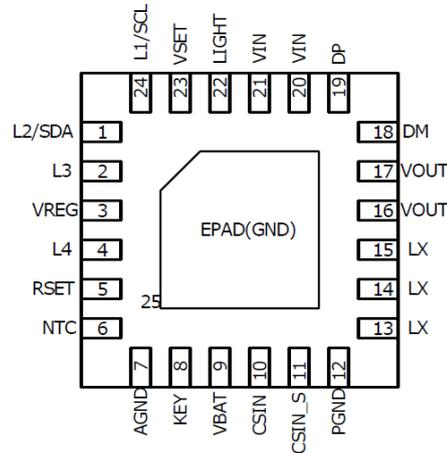
**Fig 2 IP5209 Pin Diagram**
